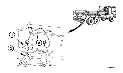
(1) Remove two pins (1) and ladder plugs (2) from ladder mounting holes (3).
