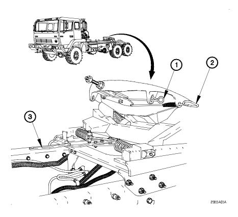
Figure 2-23. Tractor Fifth Wheel Controls
