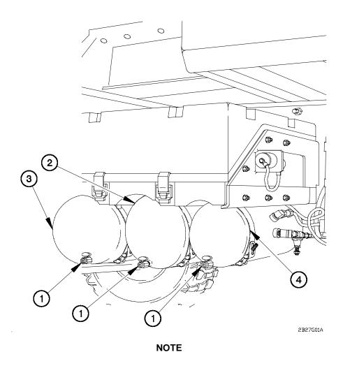
When vehicle will not be operated for 12 hours or more or when operating in temperatures below  $50^{\circ}F$  ( $10^{\circ}C$ ), air tanks should be drained.
