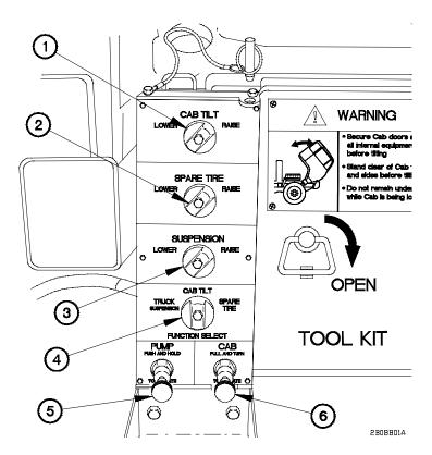
Figure 2-17. Hydraulic Manifold Controls
