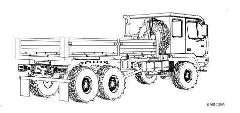
Figure 1-1. M1083 Truck, Cargo: 5-Ton, 6x6, Dropside
