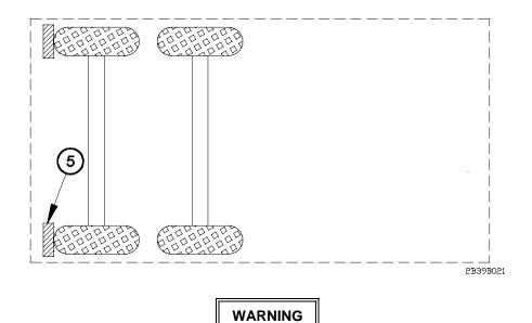
Trailer wheels must be chocked before coupling/uncoupling from fifth wheel. Trailer wheels may roll if they are not chocked. Failure to comply may result in serious injury or death to personnel or damage to equipment.
