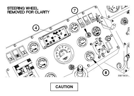
Do not engage starter pushbutton for more than 30 seconds. If engine fail s to start within this period, release starter pushbutton and wait two minut es before attempting to start engine. Failure to comply may result in dam age to equipment.
