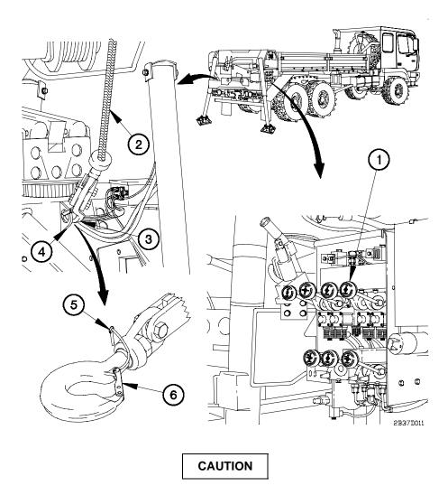
When disconnecting hook assembly from stowage ring, do not allow excessive slack to build-up when paying out cable. Cable may get tangled on drum. Failure to comply may result in damage to equipment.
