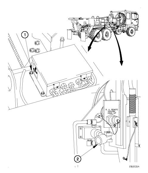
Figure 2-26. Wrecker Material Handling Crane (MHC) Controls
