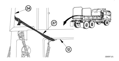
(32) Remove bow straps (37) from rear panels (12) on rear bow (34).
