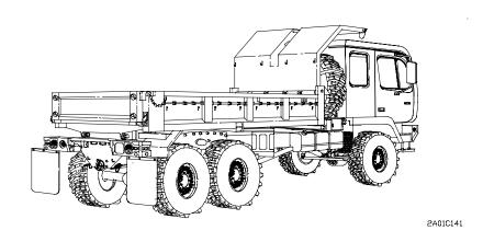
Figure 1-7. M1090 Truck, Dump: 5-Ton, 6x6
