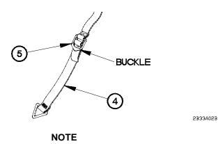
Front, center, and rear bows have two bow straps and tiedown straps. All tiedown straps are installed on bow straps the same way. One tiedown strap shown.
