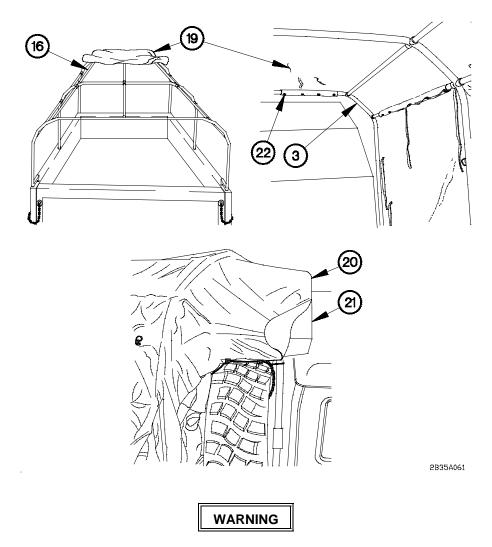
Dump cover weighs approximately 60 lbs (27 kgs). An assistant is required to lift dump cover. Failure to comply may result in injury to personnel or damage to equipment.
