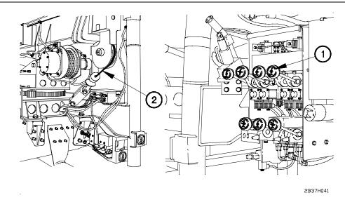
(11) Position HOIST lever (1) to UP to remove all slack from cable (2).
