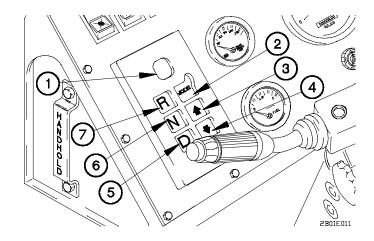
Figure 2-5. WTEC III Transmission Pushbutton Shift Selector (TPSS)
