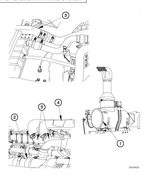
Figure 1-20. Engine Air Intake System
