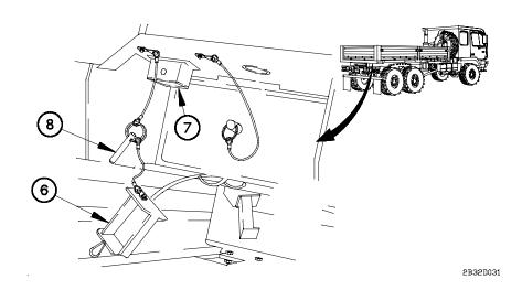
(5) Install two ladder plugs (6) in ladder mounting holes (7) with two pins (8).
