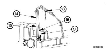
(9) Remove stowage strap (13) from front bow (14), front center bow (15), rear center bow (16), and rear bow (17).
