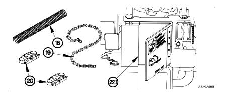
(17) Place spring (18), chain (19), and clamps (20) in tool box (22.1).
