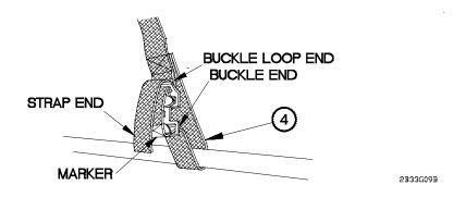
(21) Tighten left strap support (4) until marker is through the buckle end.
