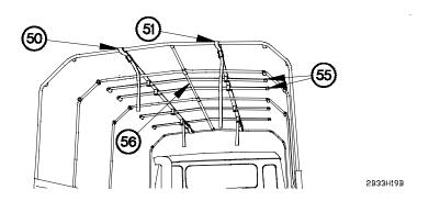
(57) Remove two braces (55) from center tube (56), left strap support (50), and right strap support (51).
