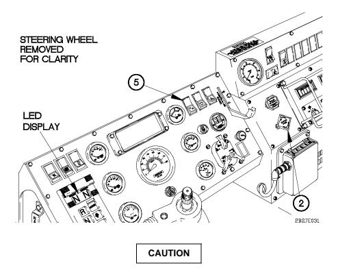
If illumination of last selected gear (in left side of LED display) goes out, WTEC II Transmission ECU Pushbutton Shift Selector (TEPSS) or WTEC III Transmission Shift Selector (TPSS) has detected a problem that needs correcting. Do not attempt to shift transmission to N (Neutral) or any other gear. Operate vehicle at reduced speed to a safe parking location. Failure to comply may result in damage to equipment.
