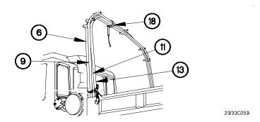
(14) Install stowage strap (18) on front bow (6), front center bow (9), rear center bow (11) and rear bow (13).
