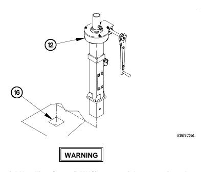
Light Material Handling Crane (LMHC) mast weighs approximately 110 lbs (50 kgs). An assistant is required to remove mast from cargo bed pocket. Failure to comply may result in injury to personnel.
