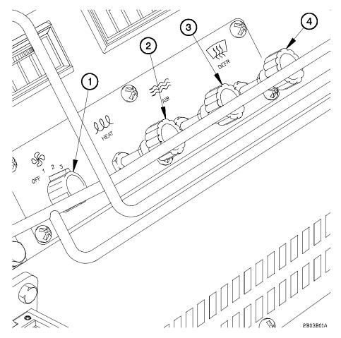
Figure 2-9. Heater/Defrost Controls
