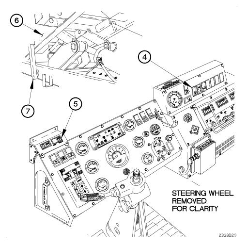
(5) Press and hold DUMP BED UP/DOWN switch (5) in UP position until dump bed (6) is completely raised.
