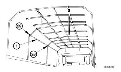
(38) Install center tube (1) in front center bow bracket (28) and rear center bow bracket (29).
