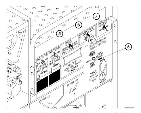
Figure 2-24. Wrecker Control Panel Fixed Operators Station (Cont)
