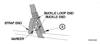
(19) Tighten left strap support (3) until marker is through the buckle end.
