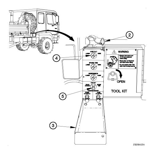
(3) Remove pin (2) from hydraulic manifold cover (3).
