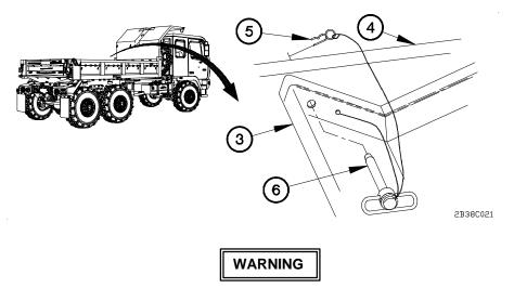
Cab protector is spring loaded and weighs approximately 180 lbs (82 kgs). Keep pressure on cab protector when lowering and when installing pins. Failure to comply may result in injury to personnel.
