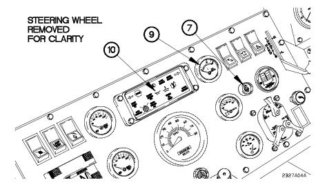
(9) Release starter pushbutton (7) when engine starts or after 30 seconds.
