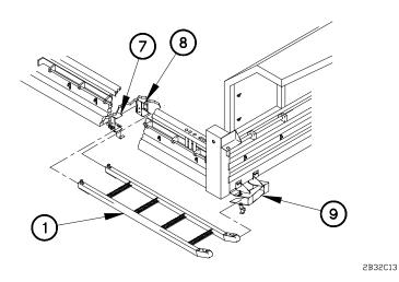
(6) Position ladder (1) in rear ladder brackets (7 and 8) and front ladder bracket (9).
