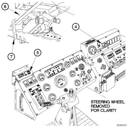
(5) Press and hold DUMP BED UP/DOWN switch (5) in UP position until dump bed (6) clears maintenance legs (7).
