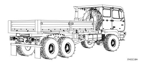
Figure 1-9. M1093 Truck, Cargo: 5-Ton, 6x6, Dropside, Air Drop
