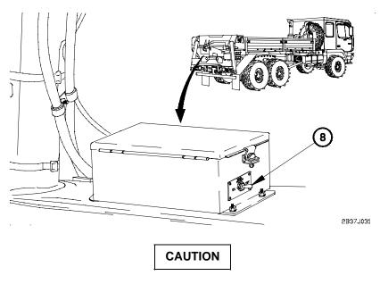
POWER ON/OFF switch must be positioned to OFF when Material Handling Crane (MHC) is not in use. Failure to comply may result in damage to equipment.
