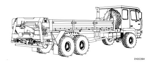
Figure 1-4. M1086 Truck, Cargo: 5-Ton, 6x6, Dropside, LWB, w/MHC
