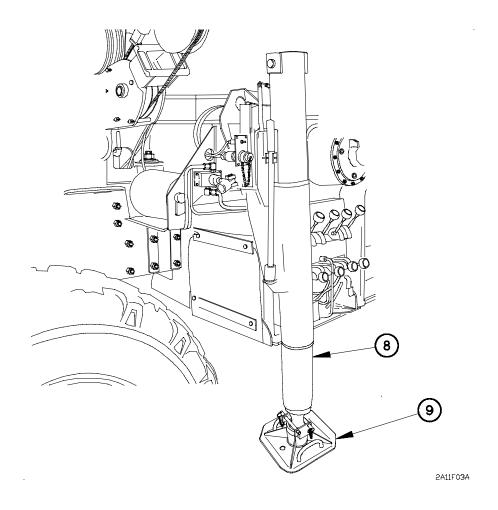
Figure 1-17. M1089 Wrecker Components Location (Cont)
