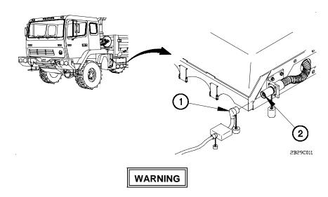
Ensure that engine is not running before disconnecting circuit breaker box NATO connector from vehicle NATO connector. Failure to comply may result in injury to personnel.
