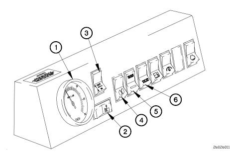
Figure 2-7. Auxiliary Panel Controls and Indicators for M1090 and M1094
