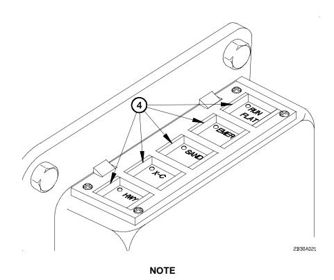
Mode light on CTIS ECU will flash when tire pressure is changing to air pressure setting for that mode. Mode light will illuminate steady when tire reaches air pressure setting for that mode.
