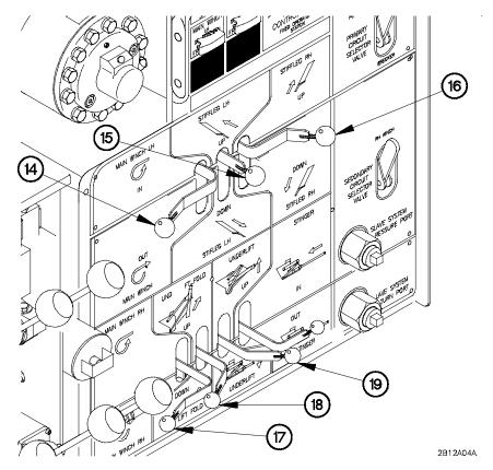
Figure 2-24. Wrecker Control Panel Fixed Operators Station (Cont)
