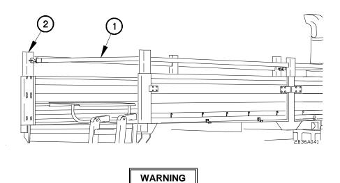
Ensure safety strap is fastened across back and front of vehicle before transporting troops. Failure to comply may result in serious injury or death to personnel.
