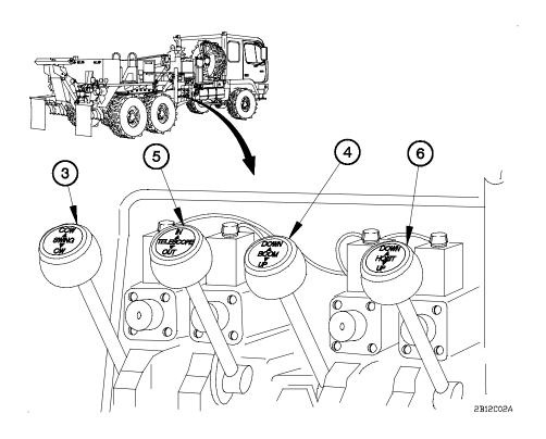
Figure 2-26. Wrecker Material Handling Crane (MHC) Controls (Cont)
