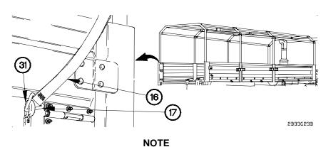
Left and right sides of front, front center, and rear center, rear bows are secured the same way. Rear bow left side shown.
