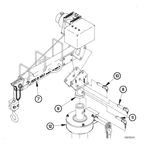
(9) Remove quick release pins (8 and 10) from turret (9).
