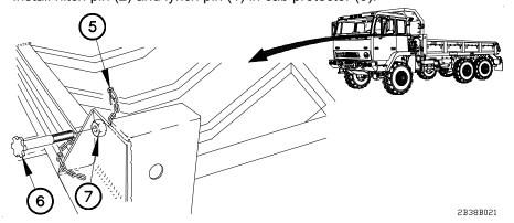
(4) Remove lynch pin (5) and turn bolt (6) from nut (7).
