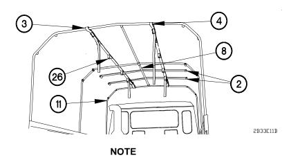
Left and right strap supports have six flaps. From front to rear of vehicle, perform step (26) on first, second, third, and fifth straps on each strap support.
