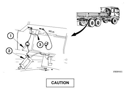
Do not use gladhands as a step to access cargo bed. Failure to comply may result in damage to equipment.
