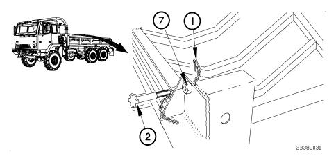
(6) Install turn bolt (2) and lynch pin (1) in nut (7).
