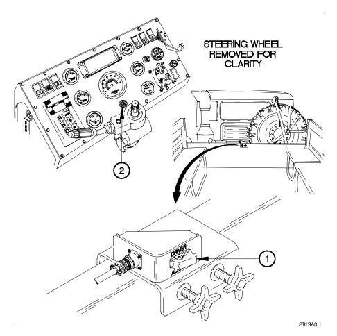
Figure 2-29. Troop Transport Alarm Switch
