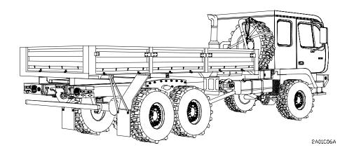
Figure 1-3. M1085 Truck, Cargo: 5-Ton, 6x6, Dropside, LWB
