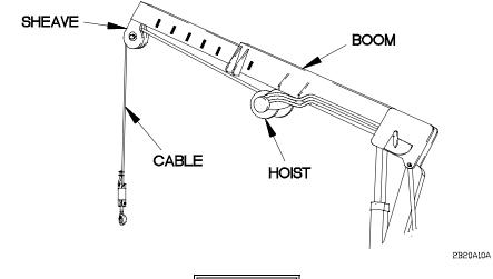
Wear heavy leather-palmed work gloves when handling cable. Cables can become frayed or contain broken wires. Never let moving cable slide through hands, even when wearing gloves. Failure to comply may result in injury to personnel.
