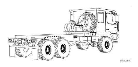
Figure 1-8. M1092 Truck, Chassis: 5-Ton, 6x6
