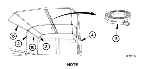
Tighten strap only enough for installation of braces.
