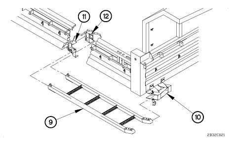
(5) Remove ladder (9) from front ladder bracket (10) and rear ladder brackets (11 and 12).
