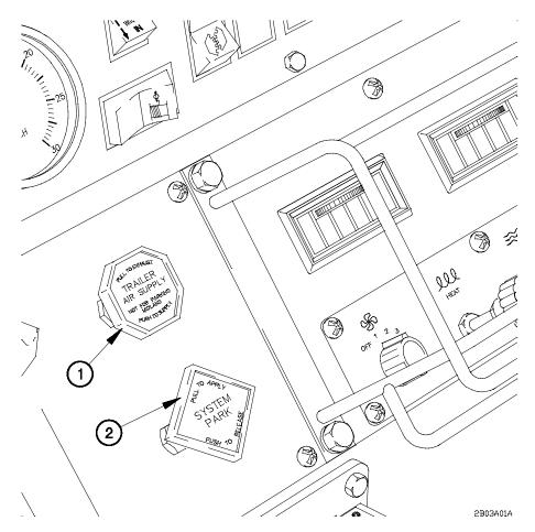
Figure 2-8. Air System Controls
