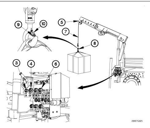
(3) Operate SWING lever (3) and TELESCOPE lever (4) to center end of boom (5) directly over load.
