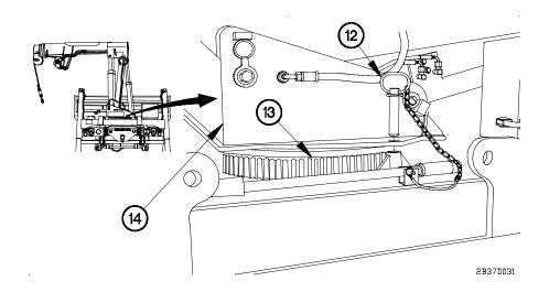
(6) Remove pin (12) from turntable bearing (13) to allow turntable (14) to rotate.
