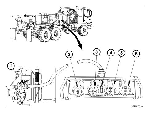
Figure 2-27. Wrecker Material Handling Crane (MHC) REMOTE CONTROL UNIT
