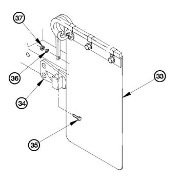
(28) Install mudflap (33) on mounting bracket (34) with screw (35), washer (36), and self-locking nut (37).
