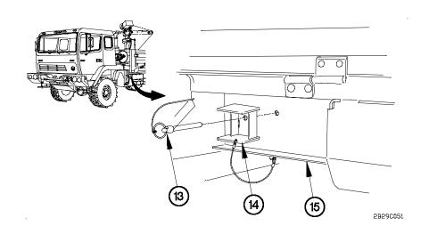
(13) Remove quick release pin (13) and plug (14) from cargo bed (15).
