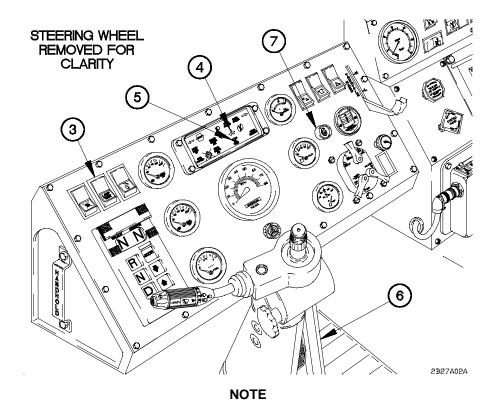
Vehicle serial number 0002 through 0017, 0019 through 0025, 0027 through 0031, 0033 through 0038, 0040 and 0041, 0043 through 0053, 0055 through 0089, 0091 through 0254, 0256 through 0258, 0260 and 0261, 0263 through 2400, and 2402 through 3091 are not equipped with Lamp Test Switch.
