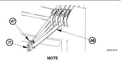
Left and right sides of front, front center, rear center, and rear bows are secured the same way. Right side shown.
