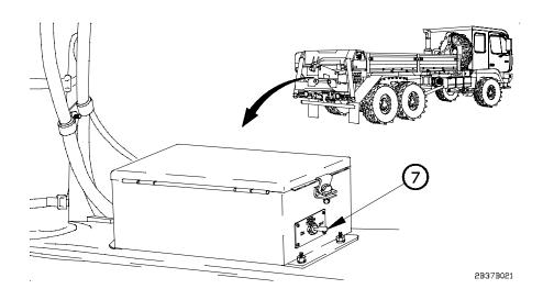
(8) Position POWER ON/OFF switch (7) to ON.
