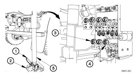
(1) Remove pin (1) from each outrigger pad (2).
