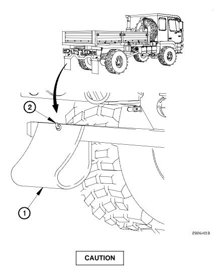
Before driving off-road, raise and hook rear mudflaps. Failure to comply may result in damage to equipment.
