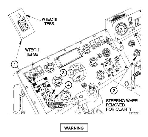
Transmission incorporates a hold feature to prohibit upshifting above selected gear during normal driving. However, during downhill operation, transmission may upshift above selected gear. On downgrades, vehicle speed may need to be restricted by using service brakes. Failure to comply may result in serious injury or death to personnel or damage to equipment.
