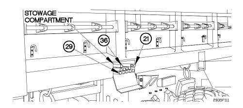
(31) Stow braces (29 and 36) and steel pole (21) in stowage compartment.
