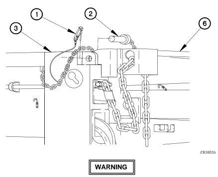
Tailgate weighs approximately 270 lbs (123 kgs). The aid of two assistants is required to raise tailgate. Failure to comply may result in serious injury or death to personnel or damage to equipment.
