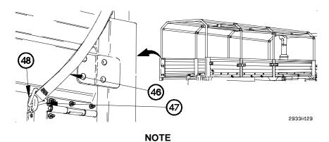
Left and right sides of front, front center, rear center, and rear bows are unsecured the same way. Rear bow left side shown.
