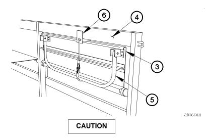
Troopseats must be stowed in the raised position when not in use. Failure to comply may result in damage to equipment.
