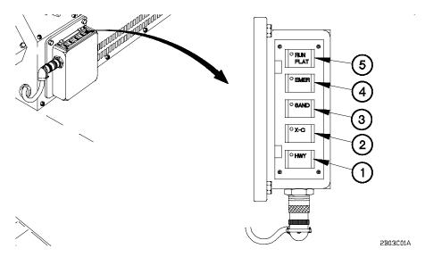
Figure 2-10. Central Tire Inflation System (CTIS) Electronic Control Unit (ECU) Controls and Indicators
