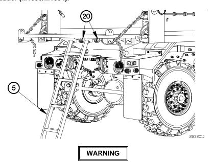
Do not press dump TAILGATE RELEASE switch while tailgate is not connected at the top. Tailgate will fall from dump body. Failure to comply may result in injury to personnel or damage to equipment.
