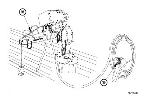
(14) To lower cable (18) place hoist control switch (19) in up position.
