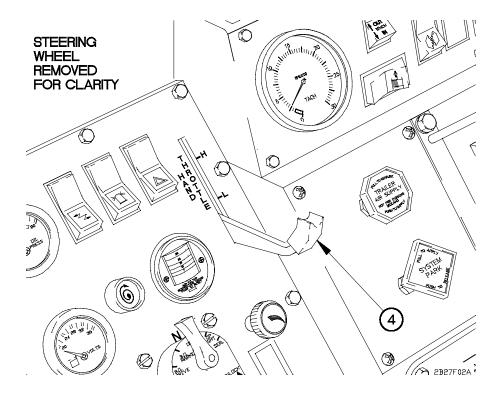
(5) Set engine to idle (750 rpm) or place HAND THROTTLE lever (4) to full down position.
