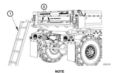
Perform step (5) to remove the ladder with the tailgate up.
