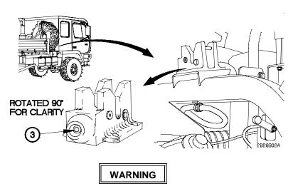
Cab hydraulic latch must be locked before driving vehicle. Failure to comply may result in serious injury or death to personnel or damage to equipment.
