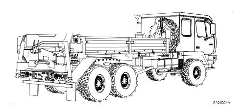
Figure 1-2. M1084 Truck, Cargo: 5-Ton, 6x6, Dropside, w/MHC
