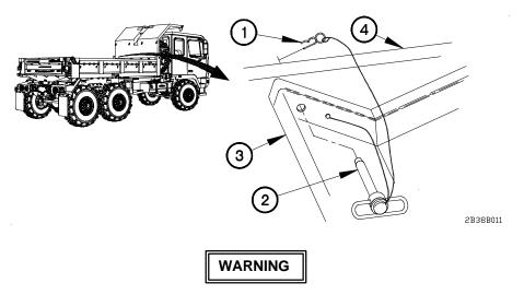
Cab protector is spring loaded and weighs approximately 180 lbs (82 kgs). Hold cab protector down before removing pins. Slowly allow cab protector to raise to upright position after pins are removed. Failure to comply may result in injury to personnel.
