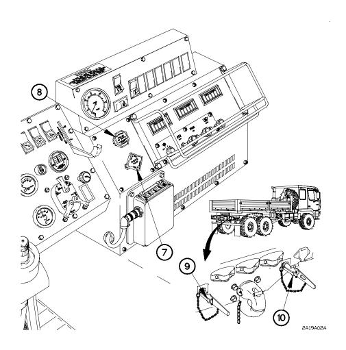
Figure 1-24. Brake System (Cont)
