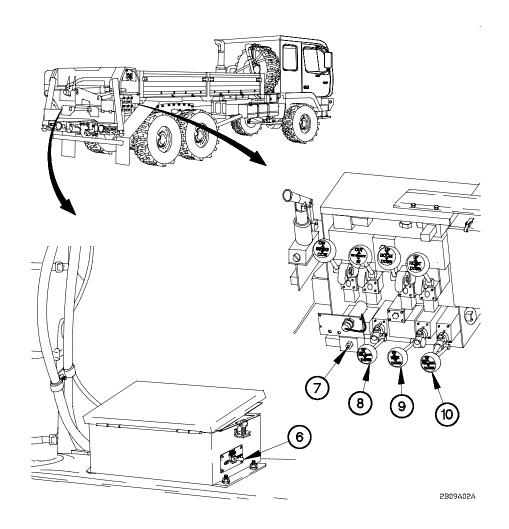
Figure 2-19. Material Handling Crane (MHC) Controls (Cont)
