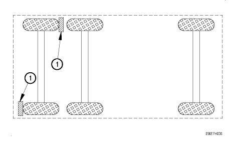
(3) Install wheel chocks (1) in front of one rear wheel and the second wheel chock in back of the opposite wheel when parked on level ground.
