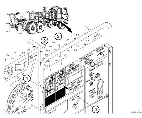
Figure 2-24. Wrecker Control Panel Fixed Operators Station
