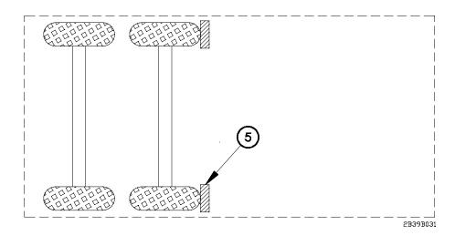
(b) Place wheel chocks (5) in front of both front trailer wheels when parked downhill.
