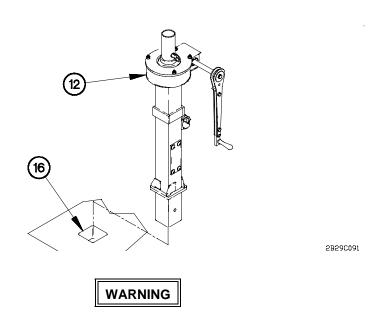
Light Material Handling Crane (LMHC) mast weighs approximately 110 lbs (50 kgs). An assistant is required to install mast in cargo bed pocket. Failure to comply may result in injury to personnel.
