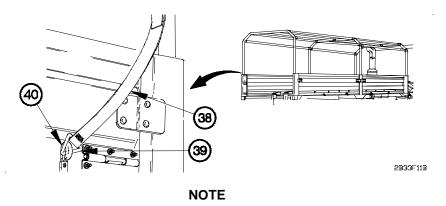
Left and right sides of front, center, and rear bows are unsecured the same way. Rear bow left side shown.
