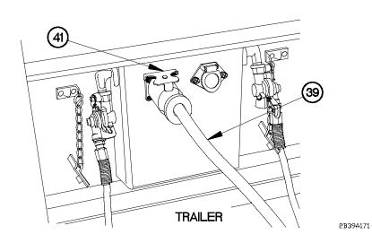
(39) Connect intervehicular cable (39) to receptacle (41) on trailer.
