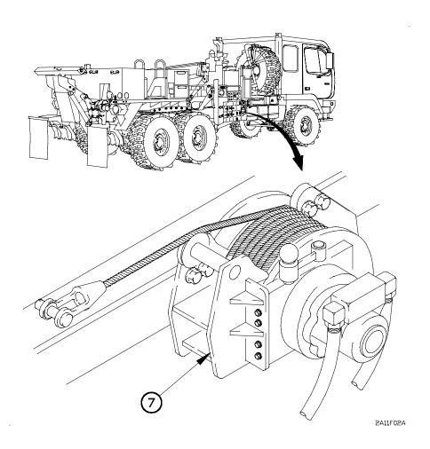
Figure 1-17. M1089 Wrecker Components Location (Cont)
