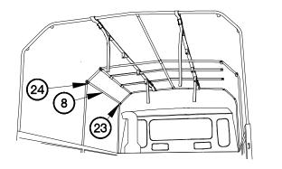
(31) Install front tube (8) in front bow bracket (23) and center bow bracket (24).
