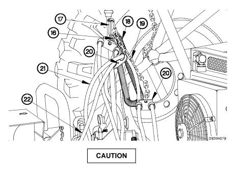
Hose clamp hook must be disconnected from snap ring before connecting to trailer. Failure to comply may result in damage to equipment.
