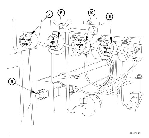
Figure 2-26. Wrecker Material Handling Crane (MHC) Controls (Cont)
