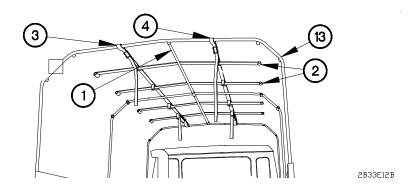
(28) Position two braces (2) over rear tube (1) and under left strap support (3) and right strap support (4) with approximately two feet (0.6 m) between rear bow (13) and each brace (2).
