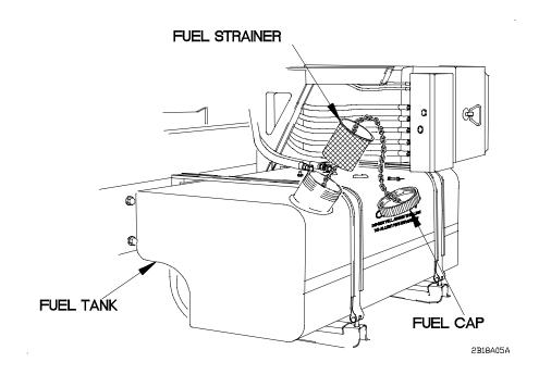
Diesel fuel is flammable. Do not fill fuel tank with engine running, while smoking, or when near an open flame. Never overfill tank or spill fuel. If fuel is spilled, clean it up immediately. Failure to comply may result in serious injury or
