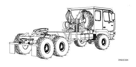
Figure 1-5. M1088 Truck, Tractor: 5-Ton, 6x6
