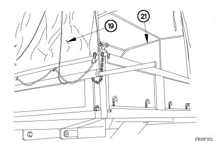
(13) Remove steel pole (21) from rear flap (19).
