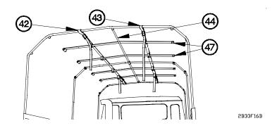
(49) Remove two braces (47) from rear tube (44), left strap support (42), and right strap support (43).
