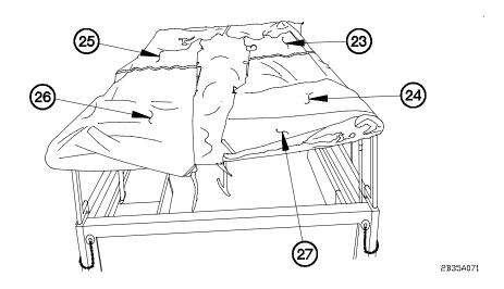
(18) Unfold right side front flap (23), right side rear flap (24), left side front flap (25), left side rear flap (26), and rear flap (27).
