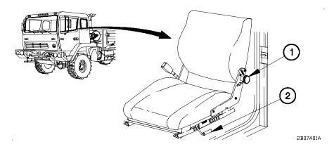
Figure 2-14. Driver's Seat Controls
