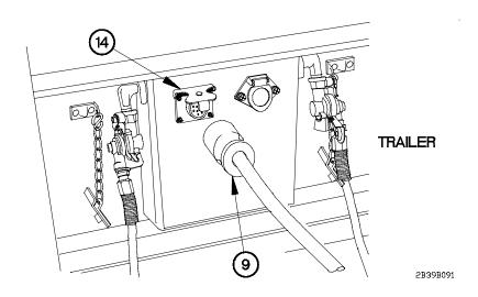
(13) Disconnect intervehicular cable (9) from receptacle (14) on trailer.
