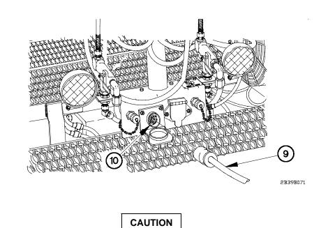
After disconnecting intervehicular cable, close the receptacle cover. Failure to comply may cause damage to equipment.
