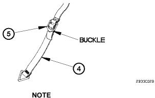
Front, front center, rear center, and rear bows have two bow straps and tiedown straps. All tiedown straps are installed on bow straps the same way. One tiedown strap shown.
