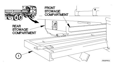
(1) Remove cargo bed side panel (1) from cargo bed stowage compartment.
