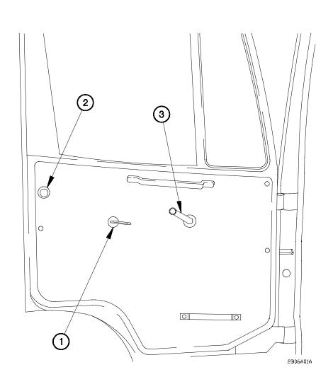
Figure 2-13. Door-Mounted Controls
