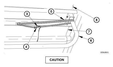
Troopseats must be stowed in the raised position when not in use. Failure to comply may result in damage to equipment.
