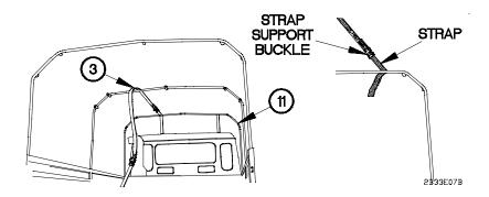
(18) Position left strap support (3) around front bow (11) and through strap support buckle.
