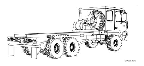
Figure 1-11. M1096 Truck, Chassis: 5-Ton, 6x6, LWB
