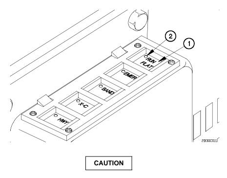
Central Tire Inflation System (CTIS) operation in RUN FLAT mode is limited to ten minutes. To continue operating CTIS in RUN FLAT mode after ten minutes, RUN FLAT mode button must be pressed again or CTIS will shut down completely. Failure to comply may result in damage to equipment.
