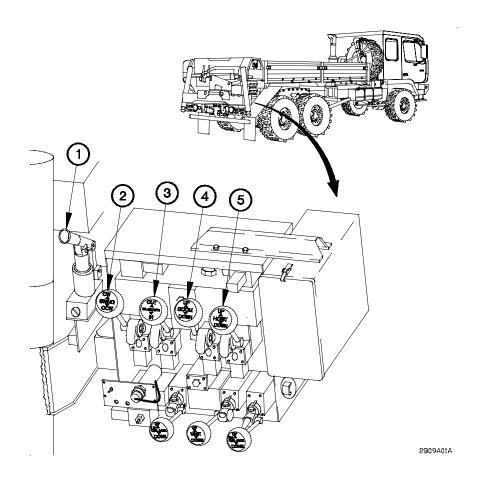
Figure 2-19. Material Handling Crane (MHC) Controls
