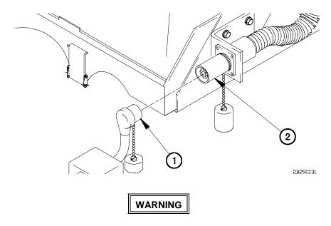
Ensure that engine is not running before disconnecting circuit breaker box NATO connector from vehicle NATO connector. Failure to comply may result in injury to personnel.
