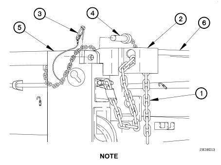
Approximately 8 chain links from chain attach point will result in 45 degree tailgate travel.
