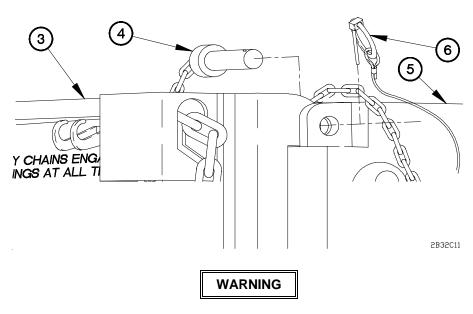
Tailgate assembly weighs approximately 270 lbs (123 kgs). Two assistants are required to raise tailgate. Failure to comply may result in serious injury or death to personnel or damage to equipment.
