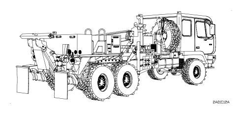
Figure 1-6. M1089 Truck, Wrecker: 5-Ton, 6x6
