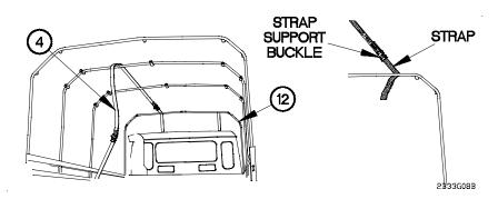
(20) Position left strap support (4) around front bow (12) and through strap support buckle.
