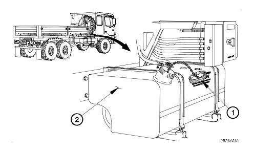
(1) Remove fuel cap (1) from fuel tank (2).
