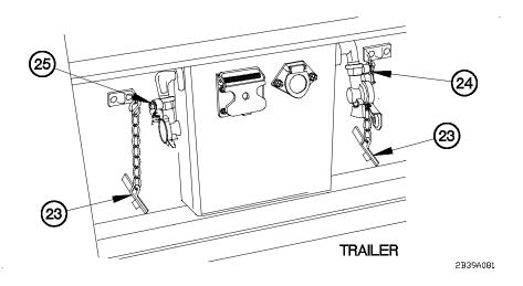
(18) Disconnect two dummy couplings (23) from SERVICE gladhand (24) and EMERGENCY gladhand (25) on trailer.
